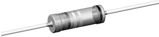
A metal glazed film is deposited on a high grade ceramic body. After a helical groove has been cut in the resistive layer, tinned electrolytic copper wires are welded to the end-caps. The resistors are coated with a light blue lacquer which provides electrical, mechanical, and climatic protection.
