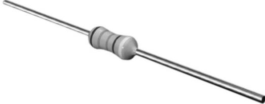
A metal glazed film is deposited on a high grade ceramic body. After a helical groove has been cut in the resistive layer, tinned electrolytic copper wires are welded to the end-caps. The resistors are coated with a light blue lacquer which provides electrical, mechanical, and climatic protection.
