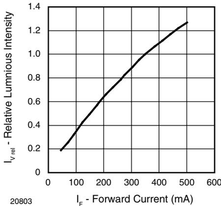
Figure 2. Relative Luminous Intensity vs. Forward Current
