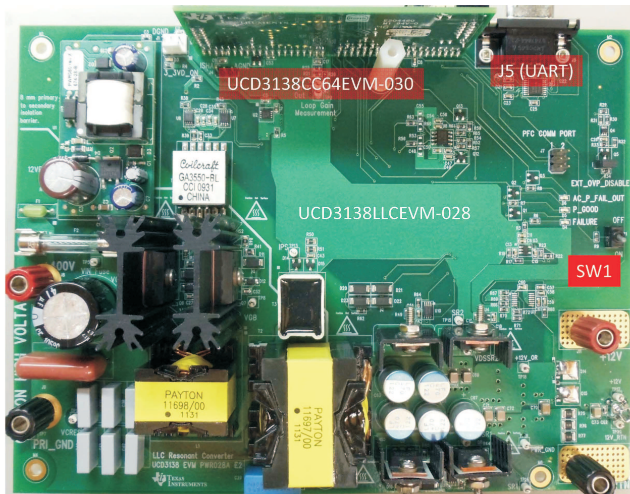
Figure 6. Orientation of Board UCD3138CC64EVM-030 on Board UCD3138LLCEVM-028
