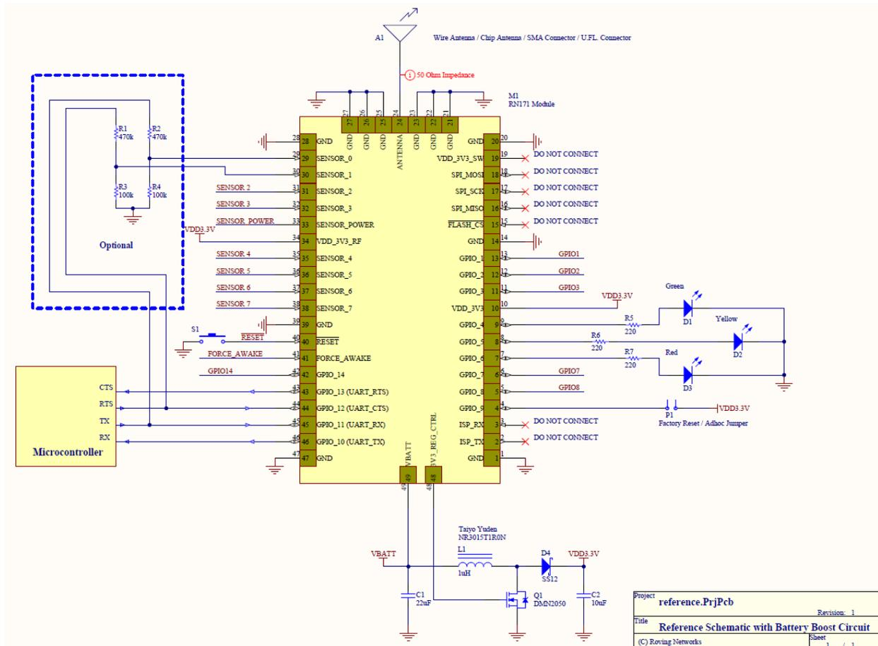
Figure 3. Typical Application Circuit with Linear Regulator
