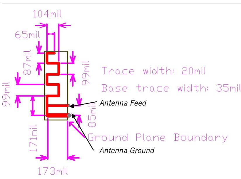
The trace from the RF pad to the antenna feed should be 12 mils thick on a 4-layer PCB to achieve 50 ohms of impedance matching as shown in Figure 7.
