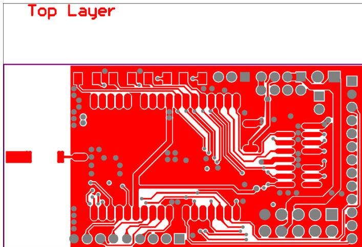
The feed connecting the antenna to the RF pad must be 50 ohm in impedance. If this feed is shorter than 0.2" the board can be 2 layers and the thickness of the feed is the same as described in the manufacturer's data sheet. If the trace is longer, you need a 4-layer board with controlled impedance, i.e., a ground plane directly under the top layer. The thickness should be calculated accordingly.
