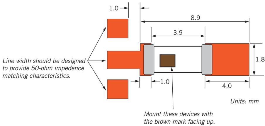
Figure 10 shows the recommended chip antenna layout.
