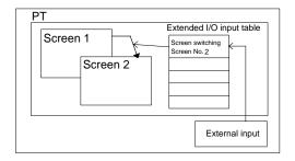
When the input terminal goes ON, the screen is switched to the set screen. If 0 is set, the display returns to the previous screen.
