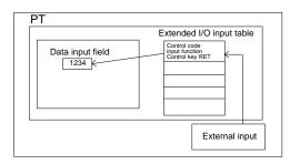
When the input terminal goes ON, it has the same effect as pressing of the control key.
