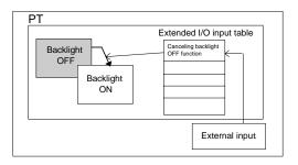
When the input terminal goes ON, the backlight, which has been turned OFF by the Cancel Backlight Off function set by a memory switch, is turned ON to redisplay the screen. A backlight OFF function releasing attribute is automatically provided for the screen switching function and the control code input function.
