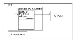
The extended I/O input table notifies the PC (PLC) of the status (ON/OFF) of the input terminals.
