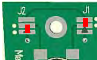
Solder pads J_1 and J_2 connection for heat flux direction (standard delivered)
