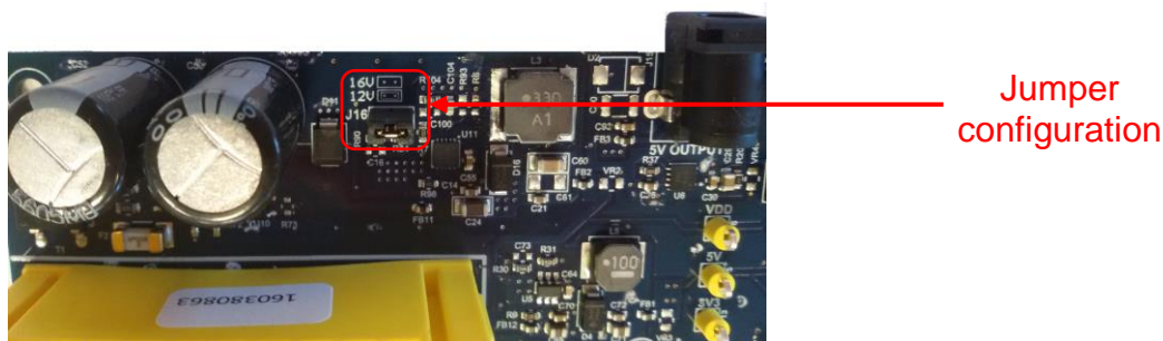
Figure 6-3. V DD selection in ATPL250ABN board.
