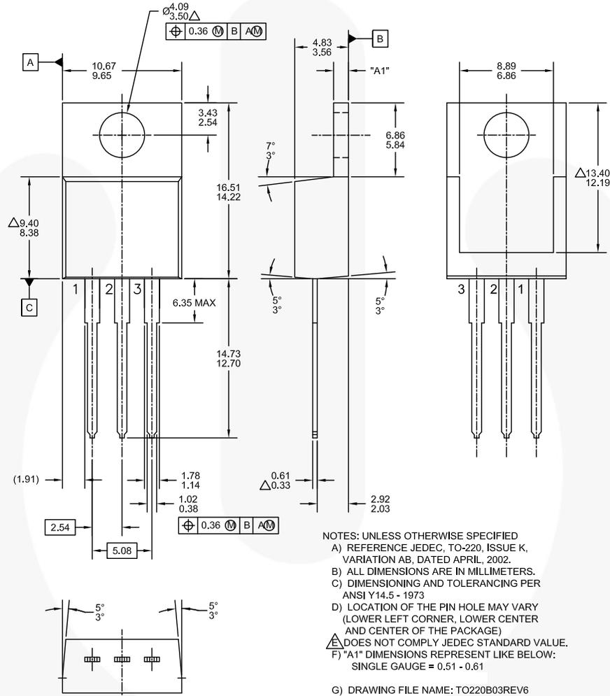
Figure 8. TO-220, MOLDED, 3-LEAD, JEDEC, VARIATION AB
