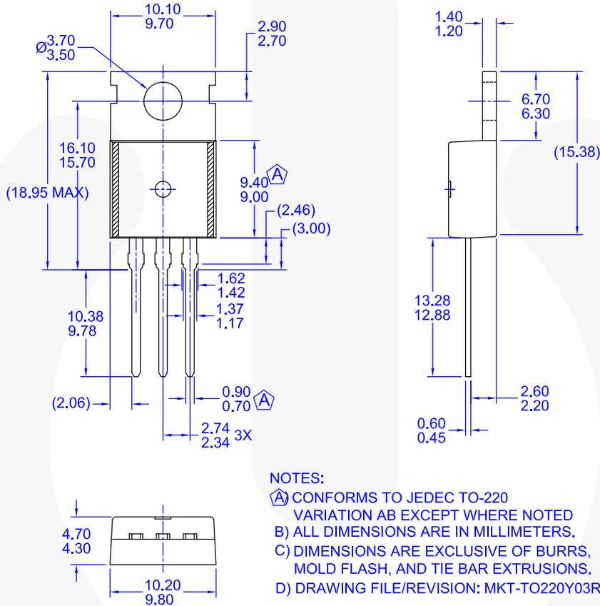
**Figure 9. TO220, MOLDED, 3-LEAD, NON-JEDEC, VARIATION AB**
