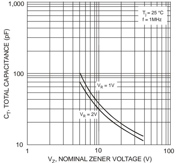
Fig. 4 Typical Total Capacitance vs. Nominal Zener Voltage
