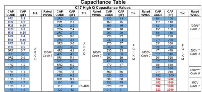
All cap values shown in **red** are available in MS only, in **blue** are available in CF, AH, and UL only. \* All CF, AH, and UL capacitors in the cap range from 110pF to 220pF are 500V rated, Code 4. \*\* All CF, AH, and UL capacitors in the cap range from 270pF to 680pF are 200V rated, Code 6. \*\*\* All CF, AH, and UL capacitors in the cap range from 820pF to 1000pF are 50V rated, Code 6.
