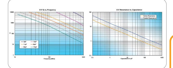
C17 **ENGINEERING KIT** CODE CAP 0.3pF 0.5pF 0.7pF 1.0pF 1.2pF 1.5pF 1.8pF 2.0pF 2.2pF 2.7pF 3.3pF 3.9pF 4.7pF 5.6pF 6.8pF 8.2pF 10pF 12pF 15pF 18pF 22pF 27pF 33pF 39pF 47pF 56pF 68pF 82pF 100pF 150pF
