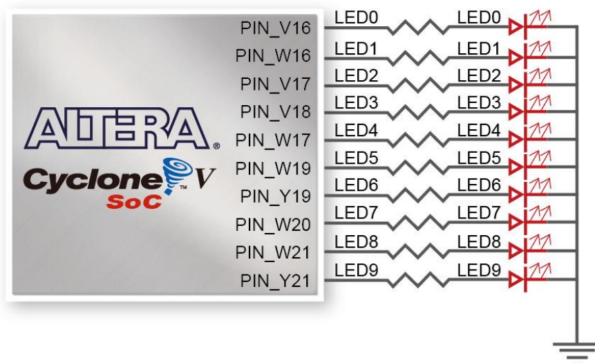
Figure 3-15 Connections between the LEDs and Cyclone V SoC FPGA
