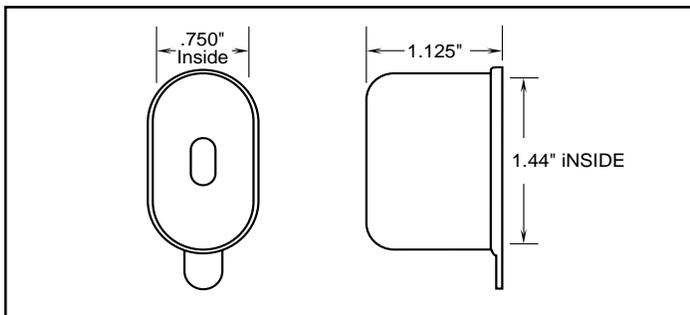
For use on capacitor types MPF/MSF, this neoprene terminal insulator, or 'boot', is used to insulate and protect the terminal area of single section units only. Material is classified 94V-1 when tested per UL94.
