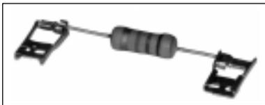
15K Ohm 2 watt bleeder resistors for AC motor start applications. Saves relay switch contacts and capacitor, particularly in capacitor start-run applications. 1/4" quick connect terminals eliminate need for soldering.
