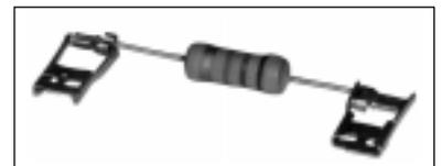
220K Ohm 1 watt bleeder resistors for AC motor run applications. Saves relay switch contacts and capacitor, particularly in capacitor start-run applications. 1/4" quick connect terminals eliminate need for soldering.
