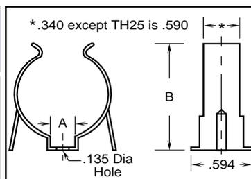
These clips, though designed for capacitors, have varied applications to retain many cylindrical components. They are used extensively in the electrical and electronic industries to hold spindles, condensers, capacitors, tubes, rods and conduit. Clips have phosphate and oil finish.
