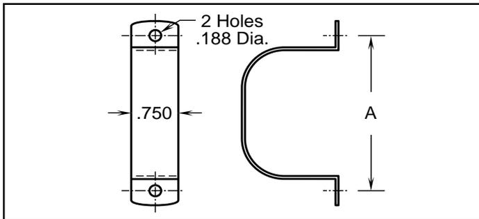
This clamp has a galvanized finish and is designed for use with the flat oval base style AC capacitors, types MPF/MSF. Material thickness is .036"
