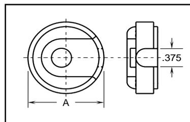
PL and PLA end caps are usually used with HB type brackets. The drawing shown at left is type PL for use with the wiring through the bracket to the motor. For off motor mounting, use type PLA. See page 214 for a photo showing a capacitor and end cap mounted in a bracket.
