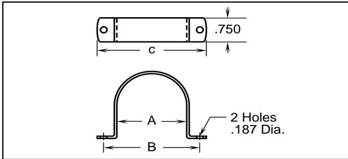
This clamp has a galvanized finish and is designed for use with the round base style motor run capacitor, types MPF. Material thickness is .035"
