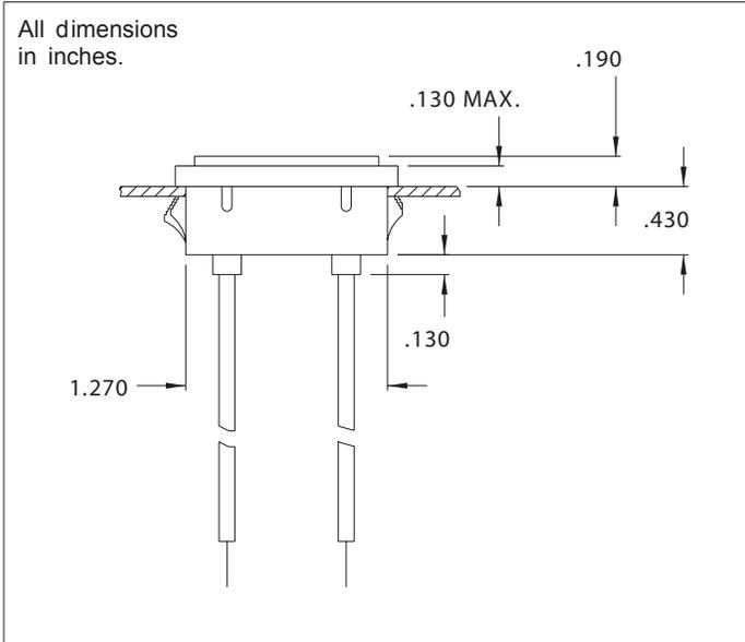
**Mounting:** Will snap-fit into  $\text{Ø}.032/.100$  thick panels. Use speednut for other panel thicknesses. Available with speednut SN1963. Mounting hole pattern on page SP3.
