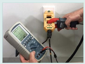
10mV/A output for use on multimeters with 1mV ACV resolution and with graphical multimeters
