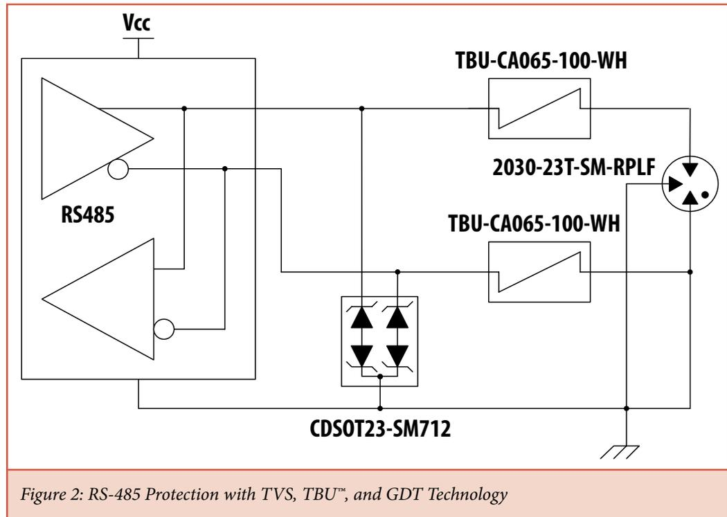
Figure 2: RS-485 Protection with TVS, TBU™, and GDT Technology
