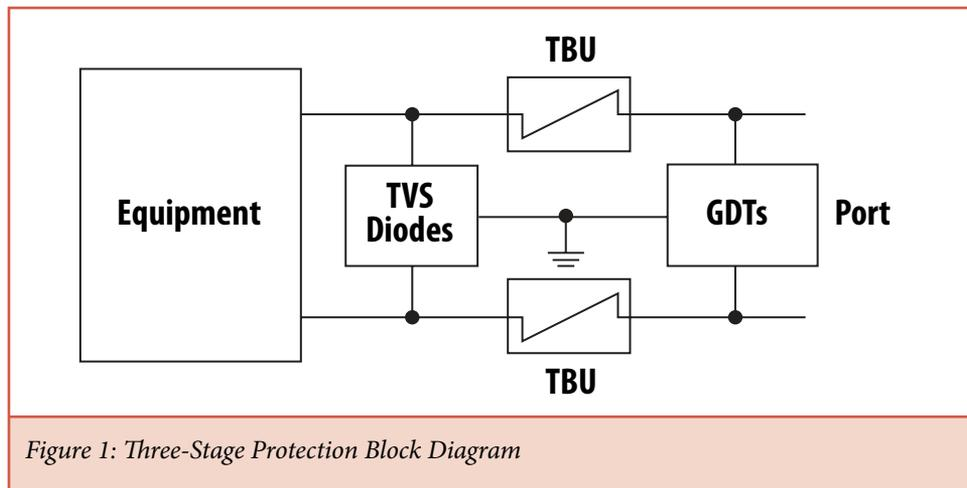
Figure 1: Three-Stage Protection Block Diagram
