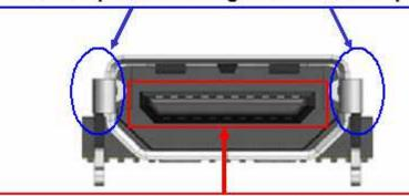
Upper row contacts are fully embedded into insulator tongue to prevent bending risk from insertion process.
