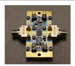
Board is 10mil thick RO4350 with 0.5oz copper cladding.
