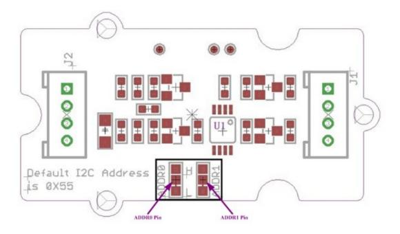
J1: used to connect Arduino IIC Interface as Grove - I2C ADC output interface.
