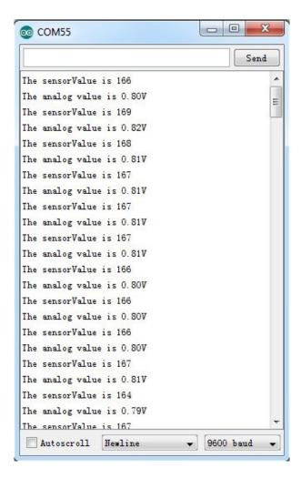
As default, Vref is generated by Arduino which is theoretically 5V. But actually that is a value afloat which results the deviation of the final data. This kind of inaccuracy is avoided when using Grove - I2C ADC, because it provides a strict 3.0V as Vref.
