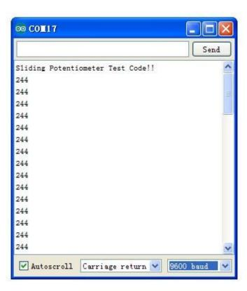
5. Move the lever back and forth. The serial data will change correspondingly. When the output resistance exceeds a certain preset value, the on-board indicator LED will also light up.
