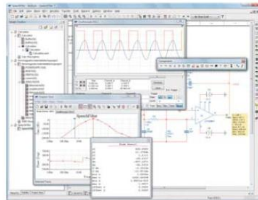
Figure 3. Use intuitive simulation instruments and analyses to validate design behavior without expertise in SPICE.
