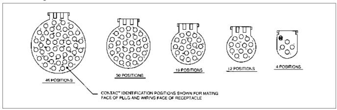
Contact identification positions shown are for mating face of plug and wiring face of receptacle.
