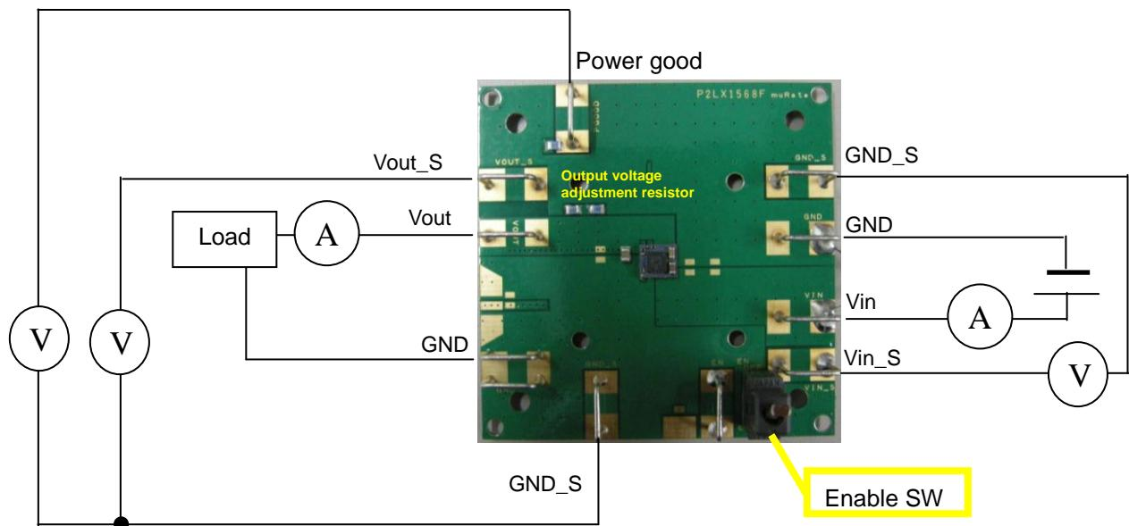
\* Evaluation board initial output Voltage setting : 3.3V (resistor : 1.3kΩ + 12Ω )
