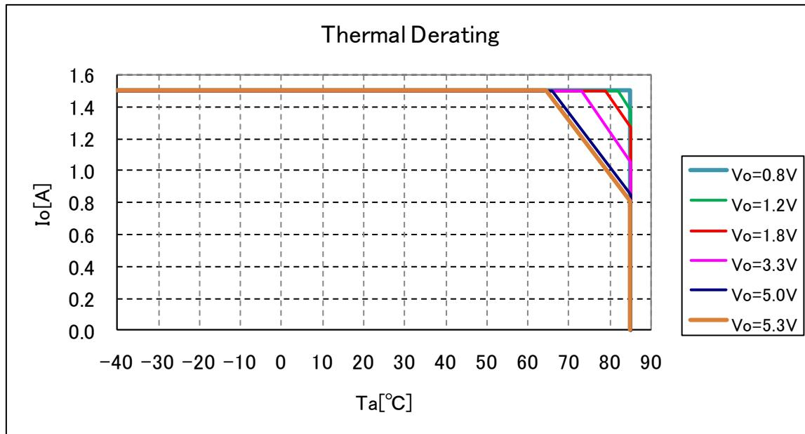
Note: This thermal derating data is measured on Murata evaluation board and reference only.
