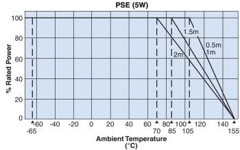
For resistors operated at rated terminal temperature a power rating shall be derated in accordance with the above derating curve.
