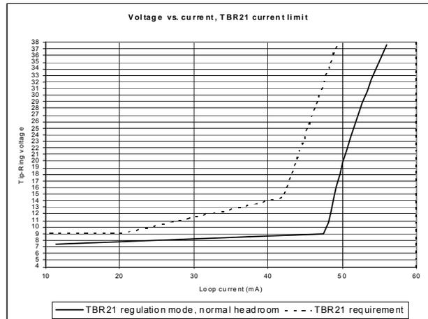
Figure 13. DC Voltage vs. Current, TBR21 Regulation
