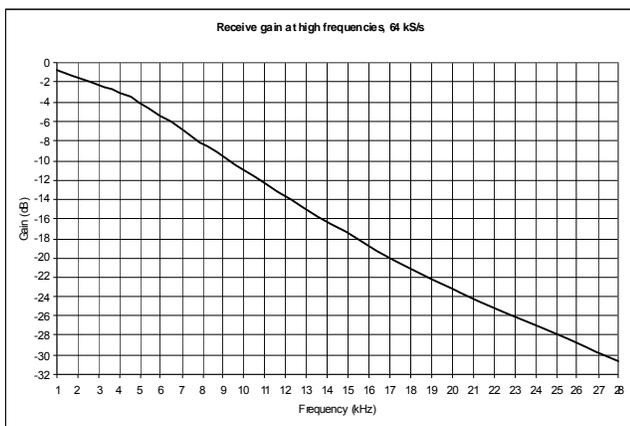
Figure 5. Receive Gain at High Frequencies (600 W)
