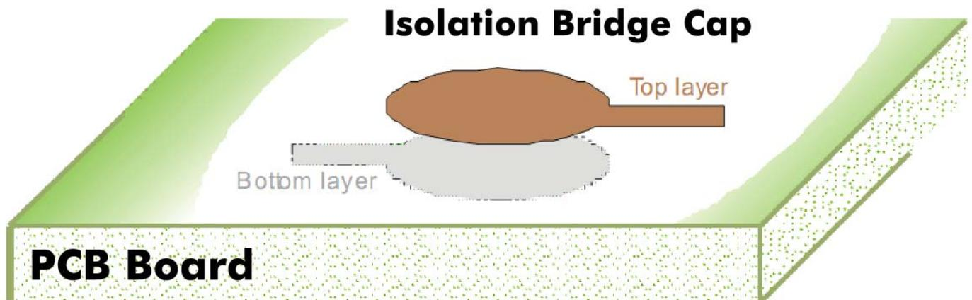
The application requires three PCB capacitors whose diameters range typically from 140 to 190 mils depending on the thickness of the board.
