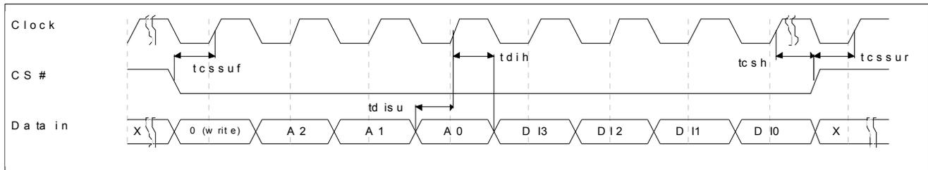
Figure 1. Serial Interface Write-Cycle Timing Diagram (Data Output Pin Floating)
