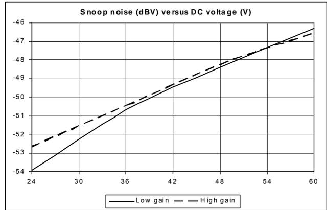
Figure 12. Snoop Noise vs. Line DC Voltage
