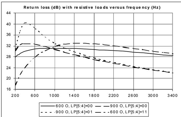
Figure 11. Return Loss for Resistive Modes
