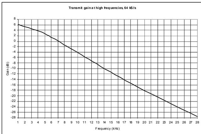
Figure 4. Transmit Gain at High Frequencies (600 Ω)
