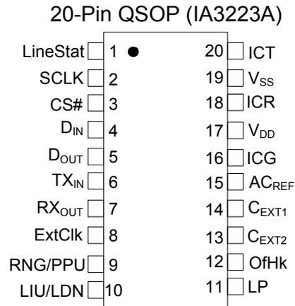
Figure 35. Pin Configuration
