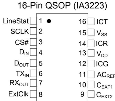
**Figure 34. Pin Configuration**
