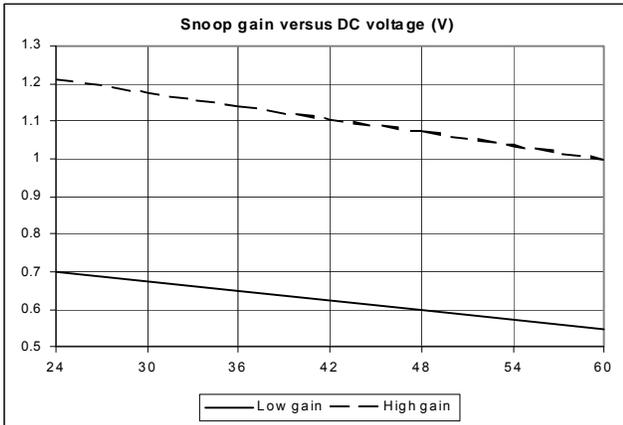
Figure 9. Snoop Gain vs. Line DC Voltage
