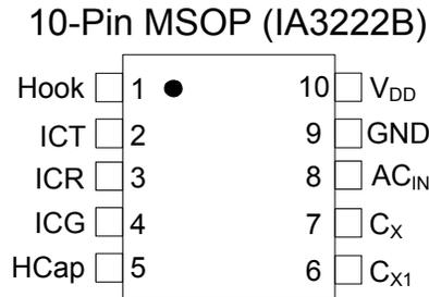
**Figure 36. Pin Configuration**
