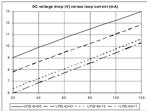
Figure 10. DC Voltage vs. Current, No Regulation
