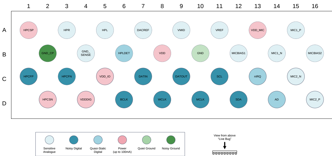
Figure 3: DA7218 Ballout Diagram
