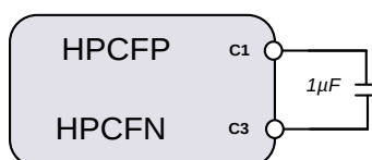
Figure 41: Charge Pump Flying Capacitor
