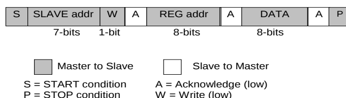
Figure 27: I 2 C Byte Write (SDA signal)
