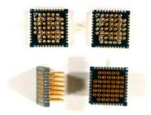
Replacement ICE Pod Feet (4) for Debugging 44-Pin TQFP PSoC Devices
