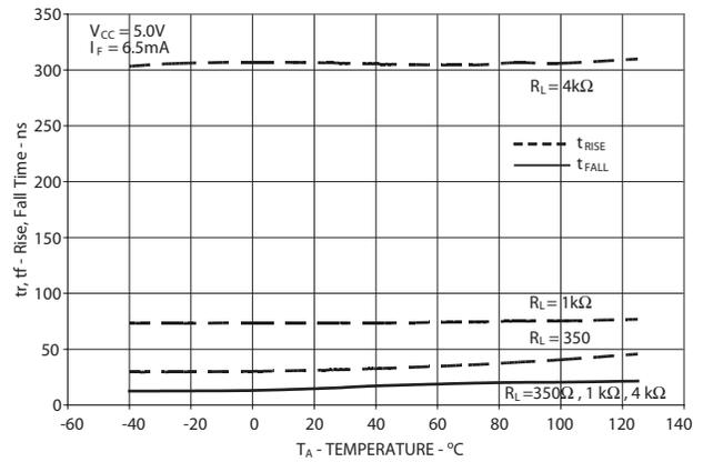
Figure 10. Rise and Fall Time vs Temperature
