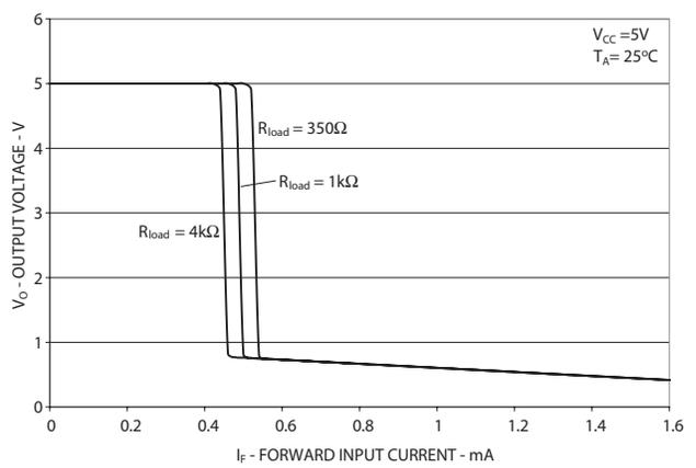
Figure 4. Output Voltage vs Forward Input current
