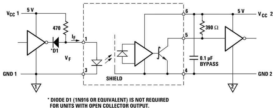
Figure 13. Recommended TTL/LSTTL to TTL/LSTTL Interface Circuit.
