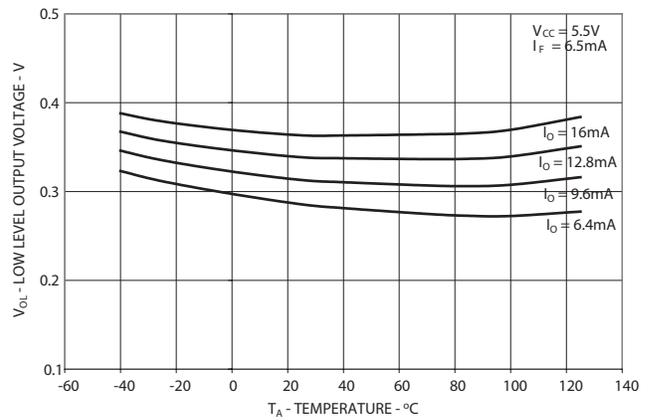
Figure 2. Low Level Output Voltage vs. Temperature
