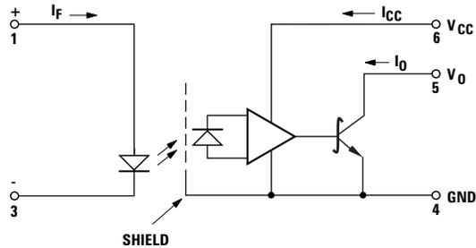
USE OF A 0.1  $\mu$ F BYPASS CAPACITOR MUST BE CONNECTED BETWEEN PINS 6 AND 4 (SEE NOTE 1).
