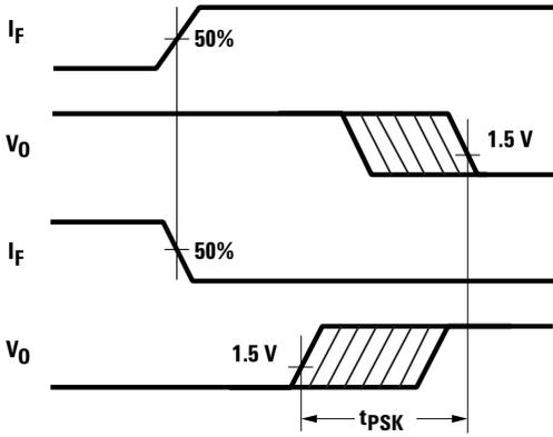
Figure 14. Illustration of Propagation Delay Skew –  $t_{PSK}$
