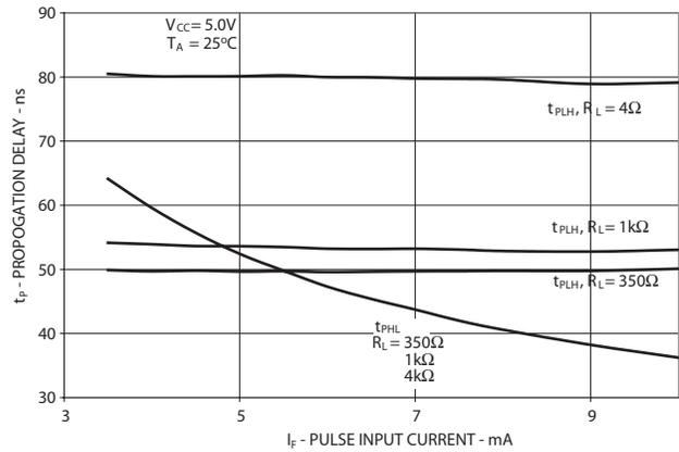
Figure 8. Propagation Delay vs. Pulse Input Current
