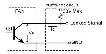
\*Transistor Q1 at "ON" position Collector current....... $I_c$ =10mA Max Saturation Voltage...... $V_{oL}$ =1.0V Max \*Transistor Q1 at "OFF" position Release Voltage...... $V_{OH}$ =30V Max
