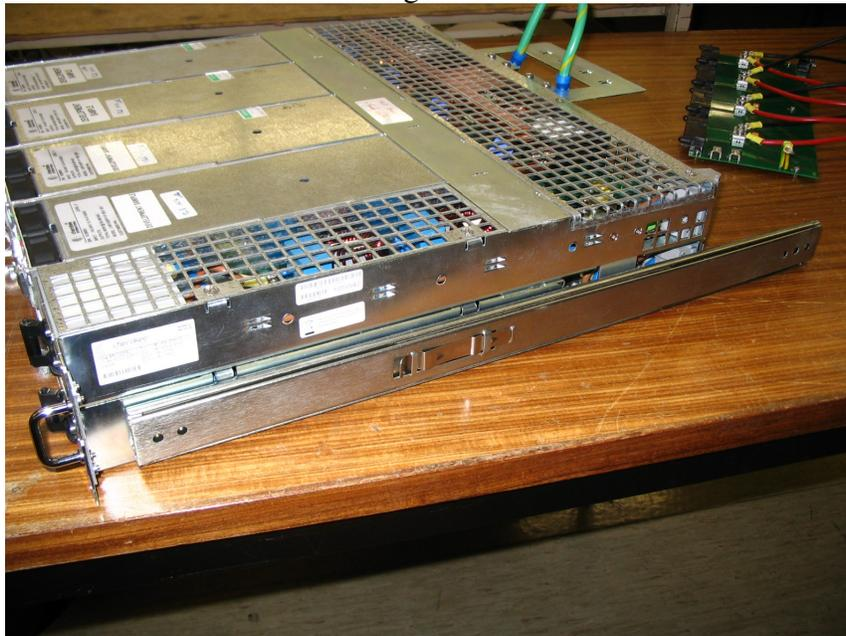
**Note:** The air inlet should not be blocked – the airflow is from front to rear.
