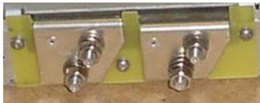
DC outputs need 2 M6 holes lugs, with 5/8 inch spacing between the centers of the holes. The lugs fixations are oblique, so the wires leave toward upper or lower side. An insulation cover is provided with the power shelf. The cover can be mounted in 2 ways following the direction of the wires.
