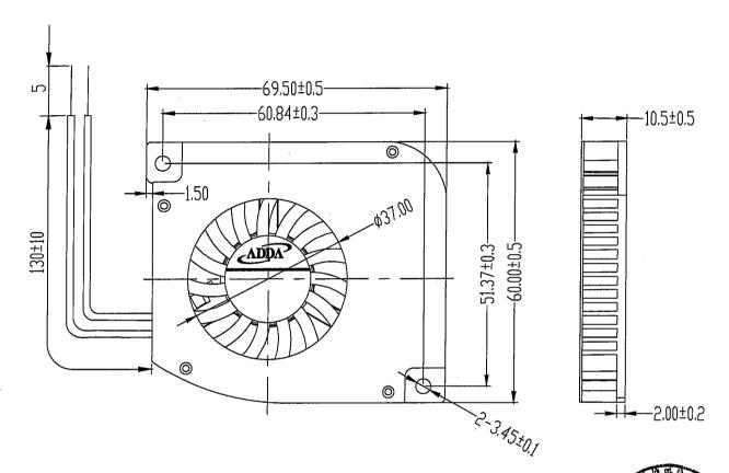
LEAD WIRES: UL 1571, AWG28, L = 130 +/- 10 mm Red = positive; Black = negative.
