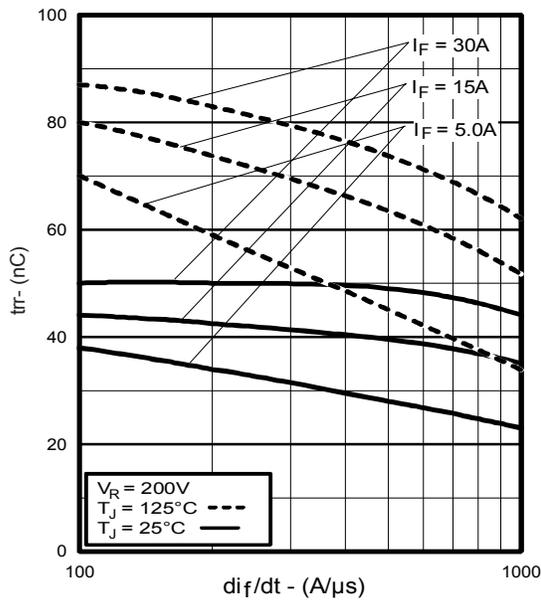
Fig. 5 - Typical Reverse Recovery vs.  $di_f/dt$
