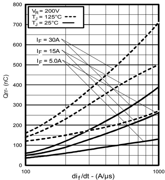
Fig. 7 - Typical Stored Charge vs.  $di_f/dt$
