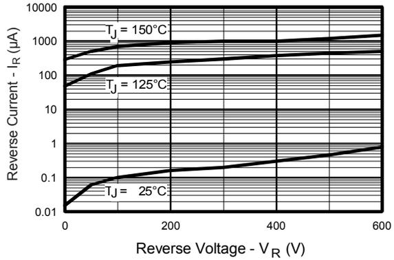
**Fig. 2** - Typical Reverse Current vs. Reverse Voltage
