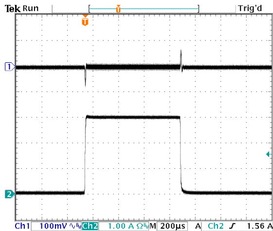
PWM Load Transient: V_{IN} = 5.0V , V_{OUT} = 1.0V Ch.1: V_{OUT} , Ch.2: I_{OUT} = 0 \leftrightarrow 3A C_{IN} = 22\mu F , C_{OUT} = 47\mu F/1206 + 10\mu F/0805
